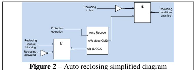
**Figure 2 – Auto reclosing simplified diagram**
