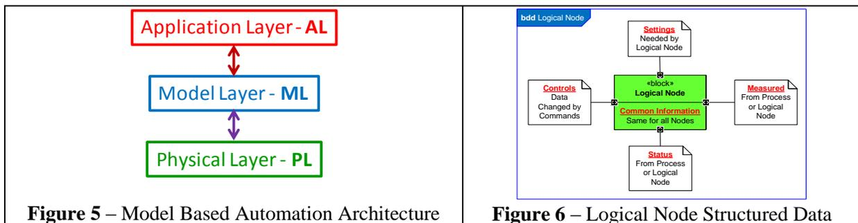
Figure 5 – Model Based Automation Architecture
