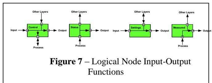
Figure 7 – Logical Node Input-Output Functions
