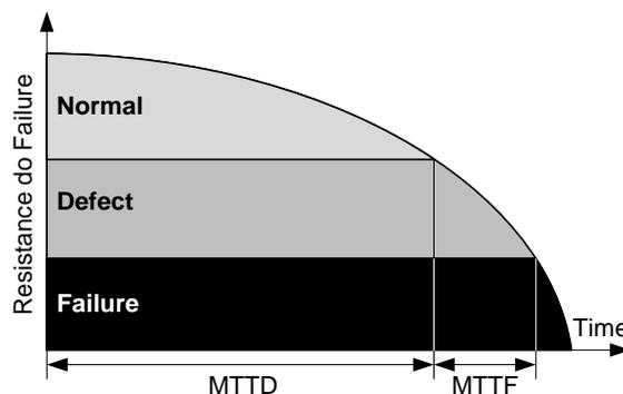
Fig. 1. IED Failure Resistance Curve
