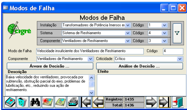
Figure 11 – Failure Mode Documentation
